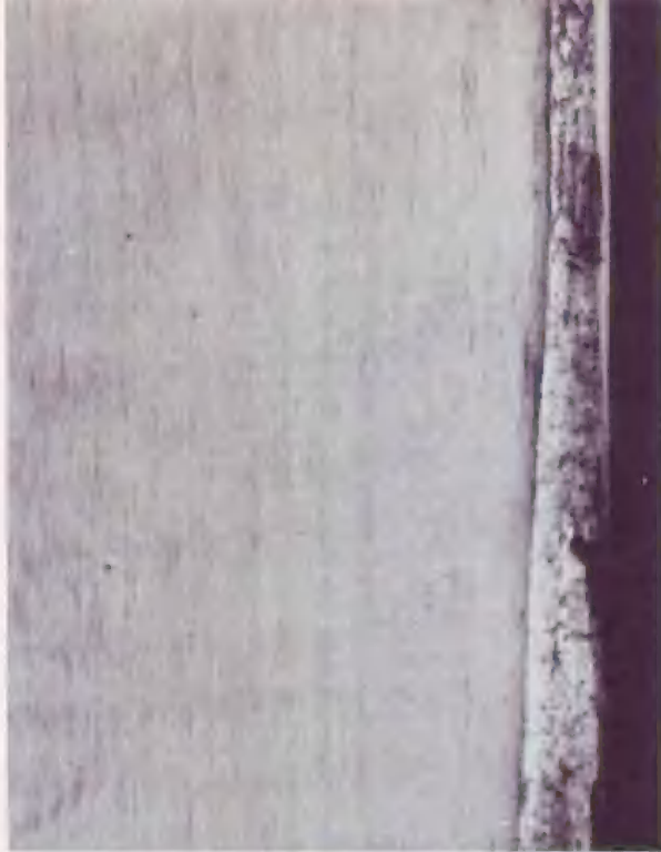
Wane: Bark or the lack of wood on the edge of the board—not eased (rounded at the edges).
